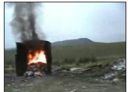
A burnbox, loaded and emptied by heavy equipment, is left open while it burns.
