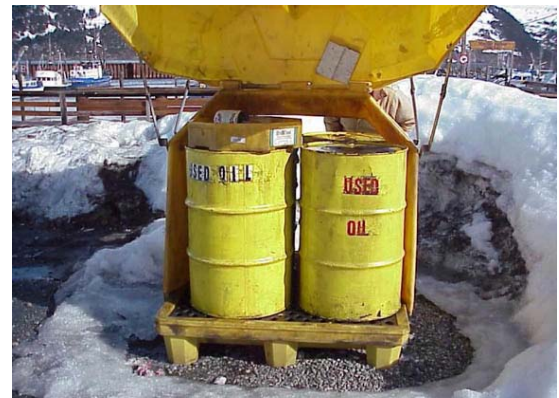
Four drum containers with spill catchment bottom and flip down lids
