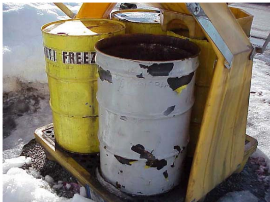
Four drum containers with spill catchment bottom and flip down lids
