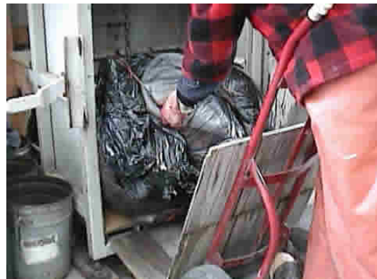
The waste bale is being ejected and is ready to go to the balefill
