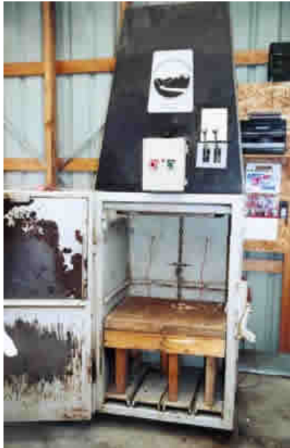
Gustavus now has two balers. This one is their original small vertical baler made by Compaction Technologies (note the wooden platform can be inserted for compacting cans etc )
