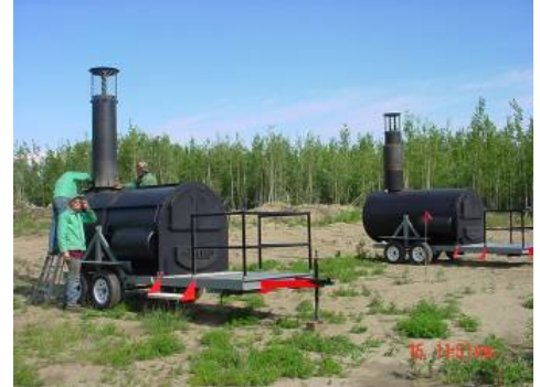
Figure 1 Conventional uninsulated unit, “Burn Unit 1” on the left and insulated unit “Burn Unit 2” on the right.
