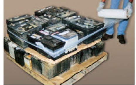
Creating a “rope-effect” with stretch wrap
