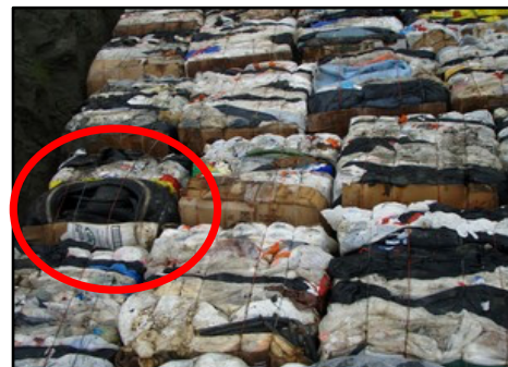
Mixed waste bale including tire from a Harmony M30HD baler in Gustavus. Bale size: 30"x24"x30"
