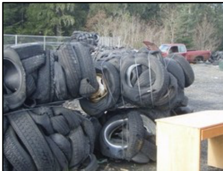
Tire-only bales from a Harris Badger baler in Petersburg. Bale size: 46"x31"x61"
