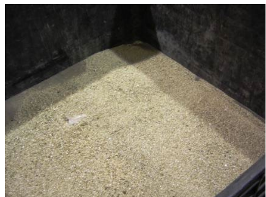
Plywood with absorbent (vermiculite) sprinkled on top
