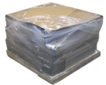
Fully wrapped pallet of batteries
