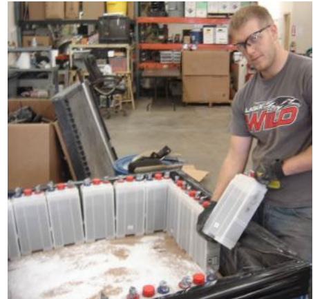
Beginning a second layer of batteries
