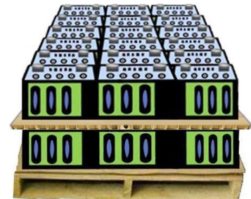
2 layers of batteries with honeycomb cardboard separating the two layers
